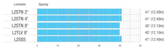
Average spacing for 1 out of every 4 luminaires, normally ON in the path of egress, when at 8, 10, or 12 foot mounting heights.
